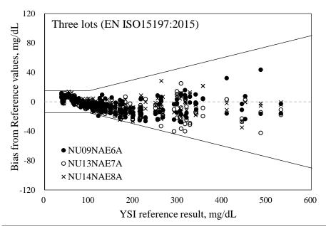
Figure 1. Premier  $\alpha$  BGMS System Accuracy Plot with Capillary Whole Blood (EN ISO 15197:2015)
