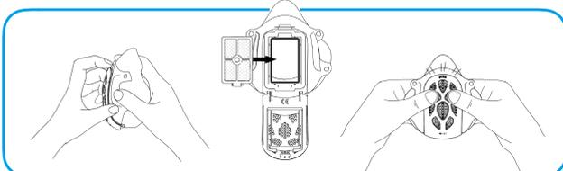
Open the door of the mask, place the cartridge inside. Make sure the orientation of the absorbent layer is correct
