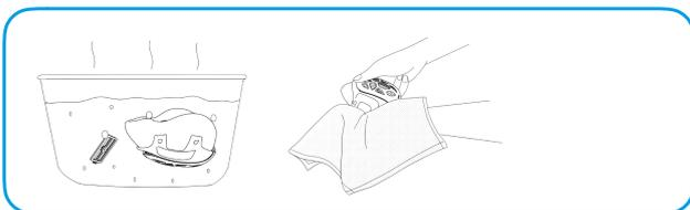
Clean the mask and cartridge by submerging them in boiling water for 2 minutes. Then let them cool and dry on a clean surface
