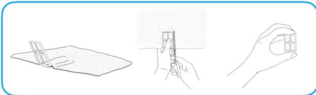
Place absorbent layer in the cartridge and hold it in place, cut out the absorbent layer
