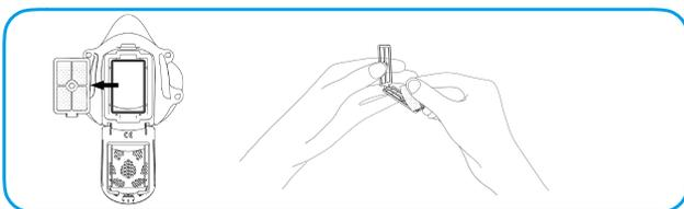
To remove the absorbent layer, open the mask door and remove the cartridge. Open the cartridge and dispose the absorbent layer
