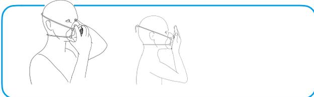
Place mask over face and adjust the strap to your comfort. Exhale air and make sure that the air does not escape from the sides of the mask
